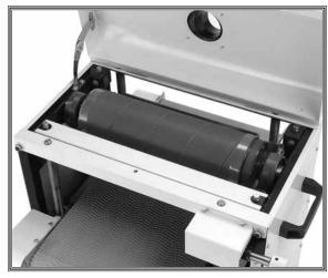
Figure 13. Sandpaper installed and taped.
